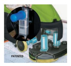
SLS (Self Levelling System) Automatic brush pressure control
